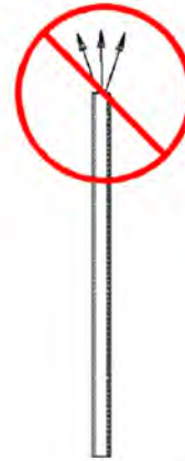
Figure 9—Example of an unacceptable vent stack that allows water accumulation
