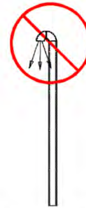
Figure 11—Example of an unacceptable vent stack that diverts gas downward; unbalanced thrust
