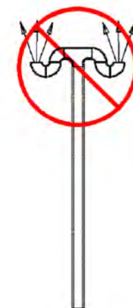
Figure 13—Example of an unacceptable vent stack with no drain holes
